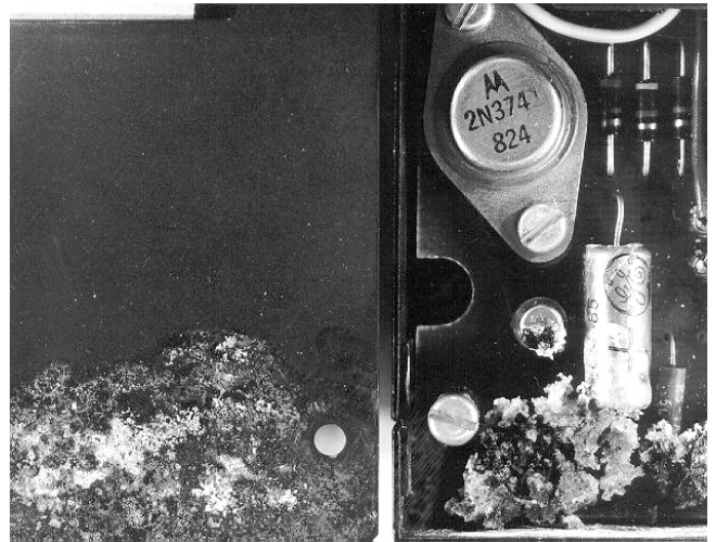
Figure 3-1. Corrosion Caused by Blown Capacitor Acid
