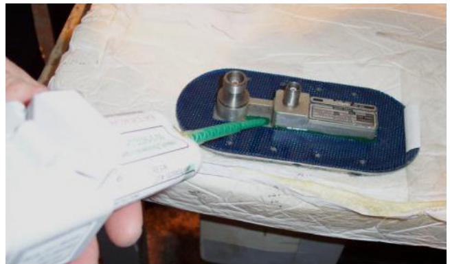
Figure 6-4. Application of Self-Leveling Green Sealant
